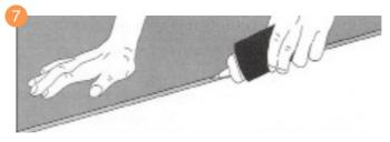
Squeeze seaming adhesive on the woven primary and secondary backings along the edge of the first piece, to prevent fraying and fibre loss. NB it is important to apply seam sealer to all cut edges.
