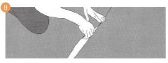
Immediately re-lay the second piece starting at the centre, press the edge into the seaming adhesive along the entire length. Any fullness of carpet should be dissipated away from the seam.
