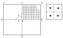
Heckmondwike FB tiles should be laid rotationally, alternating the direction of the tile through 90°. Directional arrows can be found on the reverse of each tile.
